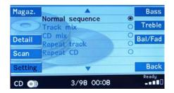
Sound controls are accessible via the three tabs at the right side of the head unit display: Bass, Treble and Bal/Fad
