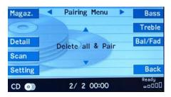
To add new device select "Pair New Device" tab then press and hold SEEK+ until the menu screen changes and hear the voice confirmation
