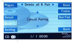
Finish pairing by entering the default pin code "0000". Paring completes with the announcement "Phone connected" and shows the signal bars
