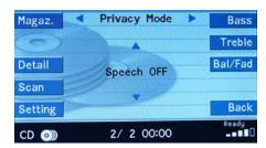
To exit without action press either any key CD1 to CD5 or press and hold SEEK- to go up one level in the menu tree
