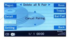
The voice will prompt to enter the access code for the phone device then pairing will be completed when the voice confirms "Phone connected"
