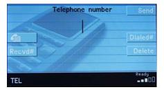
To dial type the number and then press SEND, on the bottom right screen corner the phone field strength is shown and a phone ready message
