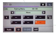
Press and hold SEEK+ to enter the Bluetooth pairing sub menu. Different pairing options are available as example "Pair new device"
