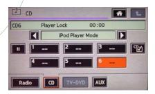
To unlock the iPod screen select the player unlock and press and hold SEEK+
