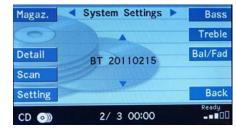
Press once SEEK+ and the screen will show a "Reset" menu. To manually reset the system press and hold SEEK+ at this step
