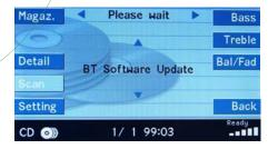
The screen will show "BT Software Update" and the track timing will show the progress 0 to 99 on the minutes and 0 to 05 on the seconds
