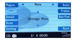
Press and hold SEEK+ key and the current software version will be displayed on the screen starting with MB
