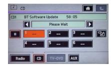
An update takes about 7 minutes. After the update is completed the head unit will reset and the screen return to the initial CD screen
