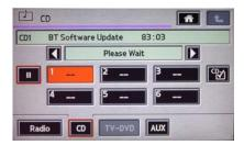
The screen will show "BT Software Update" and the track timing will show the progress 0 to 99 on the minutes and 0 to 05 on the seconds
