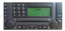
Pair the phone by searching and entering the pin. When pairing successful the coverage bars will show on the screen
