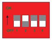
With the above switch configuration the multimedia audio will be shared with the phone function and will require typing an extra phone command
