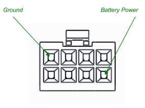
MOST 4+2 FOT Connector Plug pinout is shown below looking from the rear side.
